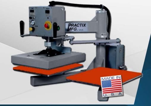
The Practix OK-25 is an automatic heavy-duty dual station swing-away tabletop press. With its large pneumatic cylinder, This machine is able to print onto materials with decreased dwell times. A quick interchangeable platen design feature is included. With it's large pneumatic cylinder, the machine is able to press onto materials with decreased dwell time.
