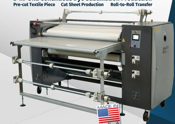
66", 88", 104" and 128" belt widths allows for heat transfer on an array of fabrics 12" dia. drum makes the OK-12 CP the fastest drum machine of class in this market
