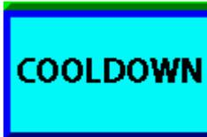
It is not necessary to move any other controls. With the machine in the "COOL DOWN" mode, the heaters are automatically de-energized with all remaining functions preserved. When the timer runs out, the machine will shut itself off completely. To restart the machine, press the HOME button to return to the HOME screen and press the START button.
