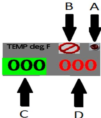
Please note that only when the belt is made operational can the heat control be activated. When the belt is not moving or during the cool down cycle, the off symbol (ITEM B) will be shown above the temperature.
