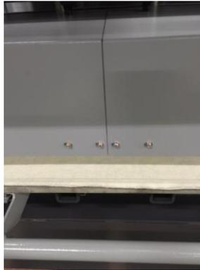
5. Remove the heater cover from the heater platen. Use care when removing the cover so that the wires are not damaged.
